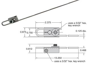
Arm: Steel 1/8" rod 13" long retained by screw clamp; the rod may be shortened and/or bent to desired shape
